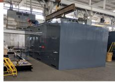
Technibus executed a project for NYC Housing Authority that included design and manufacturing of (9) LV Electrical Equipment Enclosures and (9) Sound Attenuated Natural Gas Generator Enclosures. Enclosures were manufactured from 12g A60 Galvannealed Steel. All enclosures were fabricated, assembled, integrated and witness tested at the Technibus facility.
