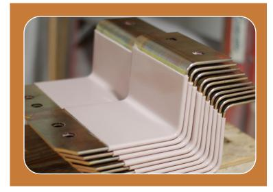
characteristics, 130°C thermal rating and high thermal emissivity are distinct advantages our insulation offers over traditional insulating products. With all of these features, our product has become the industry preference.
